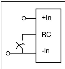
The products are fitted with a remote control function referenced to the primary negative input connection (-In), with negative and positive logic options available. The RC function allows the product to be turned on/off by an external device like a semiconductor or mechanical switch. The RC pin has an internal pull up resistor to +5 V.
