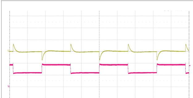
Output voltage response to load current step-change (0.278-0.416-0.278 A) at:
