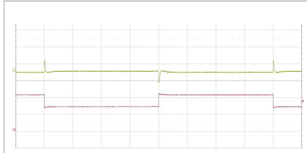
Output voltage response to load current step-
