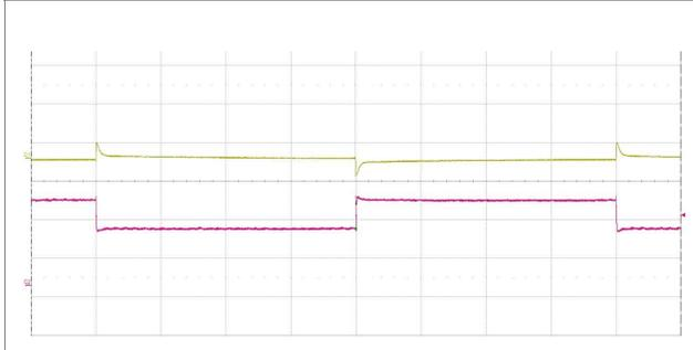
Output voltage response to load current step-
