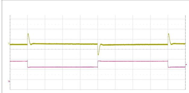
Output voltage response to load current step-
