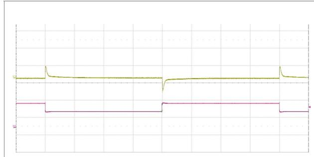
Output voltage response to load current step-
