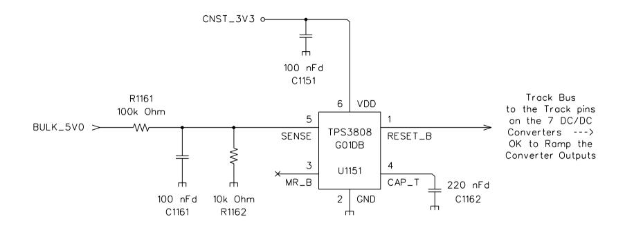
The 10k Ohm and 100 nFd provide about 1 msec of filtering.
