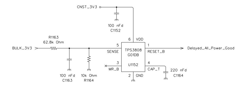
The 10k Ohm and 100 nFd provide about 1 msec of filtering.
