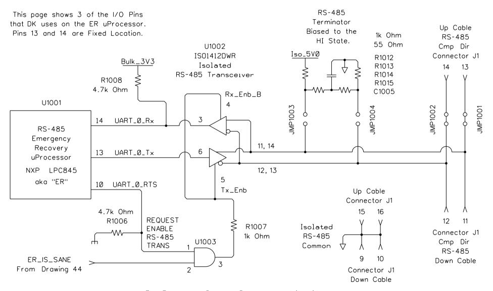
The Emergency Rescue uProcessor and its side of the RS-485 Transceiver are powered by Bulk\_3V3.
