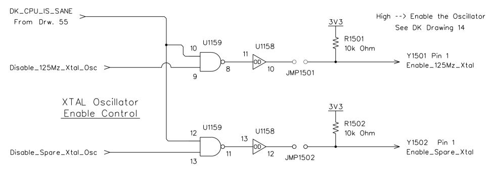
HI Active Disable signals from the DK's CPU GPIO
