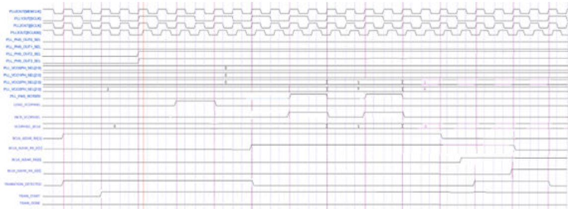
Figure 11-14. BCLK90(Clk) SCLK(Dat)—Transition Detection
