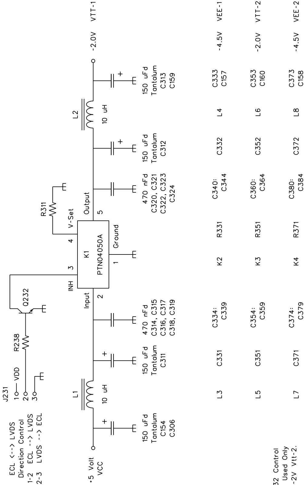
The Q232 Control Circuit Is Used Only with K3 -2V VTT-2. Pin #3 on K1, K2, and K4 Is Floating.
