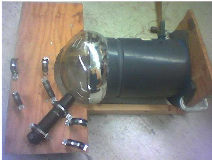
Figure 1: PMT and light source support structure
