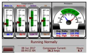
The "All Inputs" screen is designed to give the user a complete picture of all the temperatures and pressures being monitored by the system. The Coolant In & Out icons will change depending on the system attached. The pressure readings are a result of averaging data over a 20 second period. If the compressor has an inverter, inverter current and frequency information is also displayed on the left of the screen along with detected cryocooler RPM. This RPM is detected via gas pulses.
