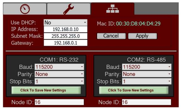
This page shows the IP data that gets assigned to the device by its network. By connecting to the compressor via serial port or by Ethernet it is possible to remotely monitor and operate the compressor. Compressors with a single DB-9 port only support RS-232. Compressors with two DB-9 ports also provide an RS-485 port.
