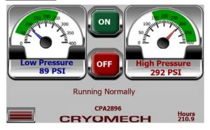
The left dial indicates the low or gas input pressure and the right dial indicates the high or output pressure. Status about the running state of the compressor will be displayed on the Feedback Label. The bottom right Hours number tracks the total hours of operation the compressor has been running.
