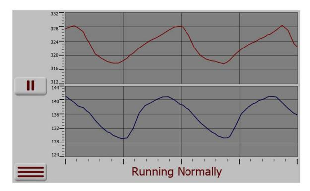
The pressure monitoring mode has a time span of 2 seconds. The high and low pressures scales are independent and auto adjust based on captured data. A pause button is provided to allow closer examination of the charts.
