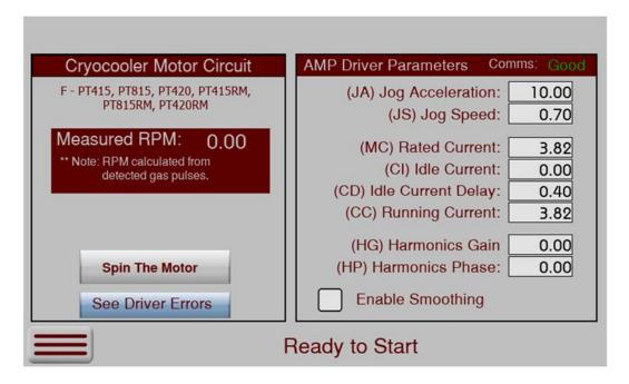
This screen allows inspection of the parameters used to operate the cryocooler. Note the Amp Driver Parameters only properly update while the system is not running. Smoothing can be used to try and reduce the amount of motor vibration in the cryocooler.
