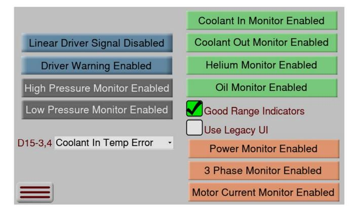
This screen allows the operator to disable a single sensor, the sensor may be ignored allowing the compressor to run until such time that the sensor can be replaced. This is also where the use of Legacy UI can be enabled. The Good Range Indicators only applies to temperature scales in the Legacy UI format.
