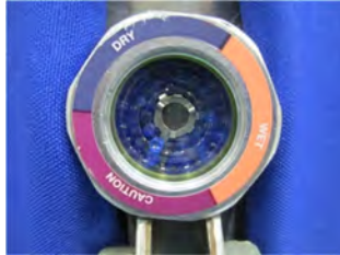
Figure 7-3a: Blue beads signify a dry condition.
