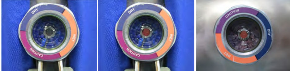
Figure 8-6a: Blue beads signify a dry condition.
