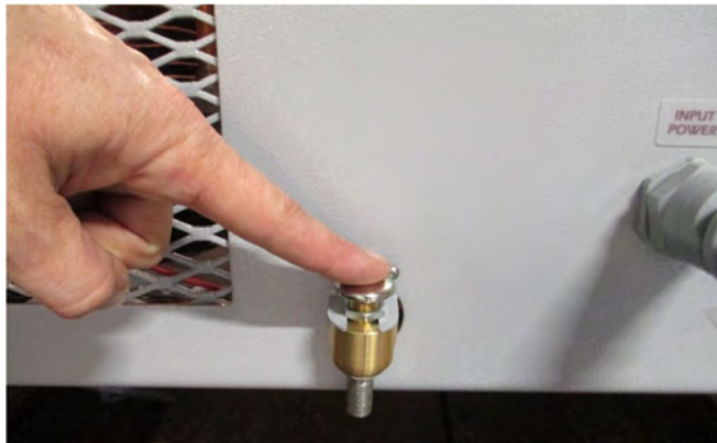
Figure 8-11: H 2 O Drain Valve
