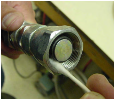
Figure 1 Cleaning the female Aeroquip®
