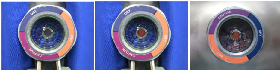
Figure 8-4a: Blue beads signify a dry condition.
