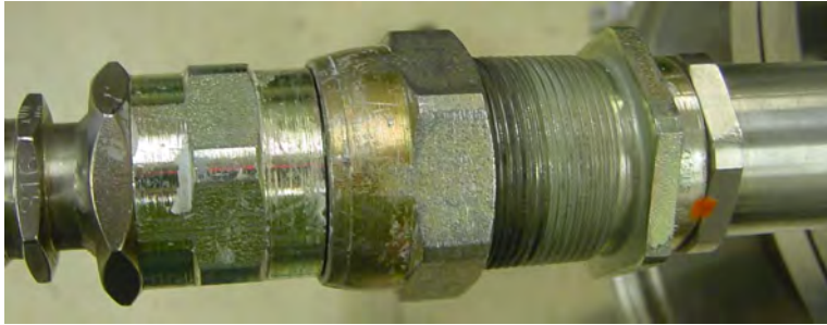
Figure 3 Female to male connection, hand tightened
