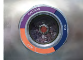
Figure 7-3c: Pink dot and pink beads signify an oversaturated adsorber. Regenerate adsorber.
