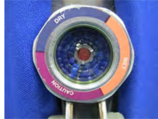
Figure 7-3b: Pink dot signifies a saturated adsorber. Regenerate adsorber.
