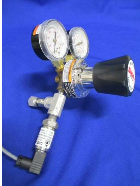
Figure B-2: Pressure regulator at storage cylinders
