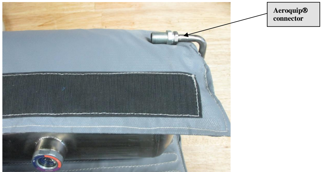
Figure D-9: Heating jacket, containing adsorber
