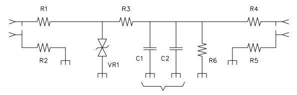
Good Ground Connection to the Filter Box and through the Filter Mounting Bracket to the Cryostat.
