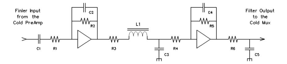
The Drift Velocity is 1.5 mm/usec in a 500 V/cm field. For a 3 to 5 mm plane spacing the risetime will be 2 to 3.3 usec. For now pick a 2.5 usec peaking time or about 64 kHz.
