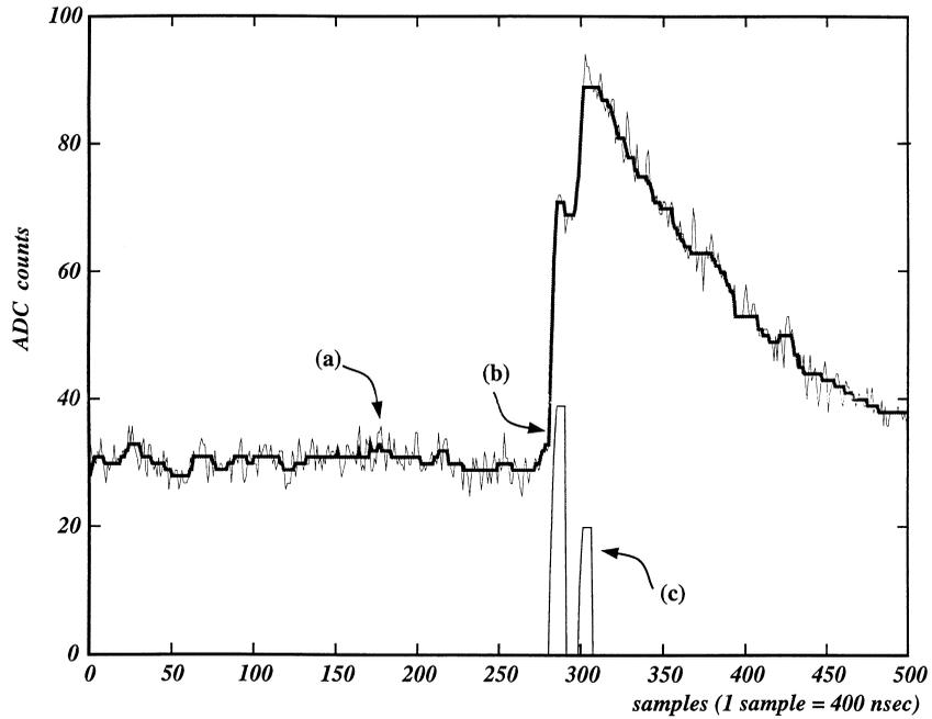
Fig. 1. Icarus collection signal before (a) and after (b) median filtering; Daedalus filtered output (c).
