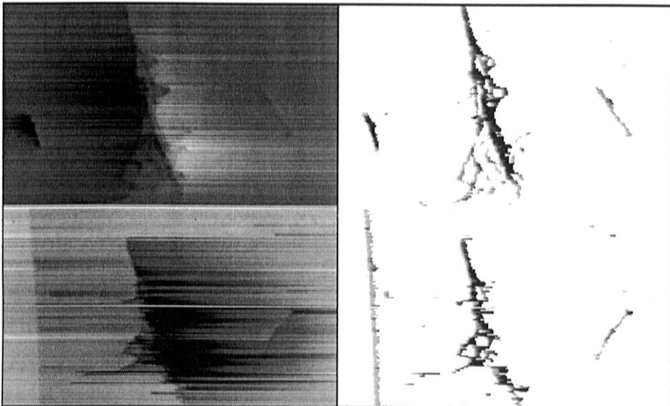
Fig. 2. Collection and induction image of an Icarus event before (left) and after (right) filtering.
