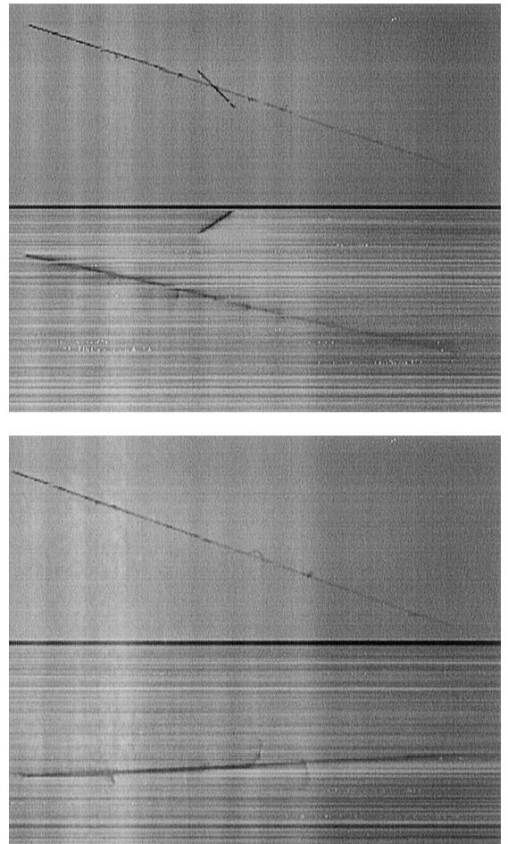
Fig. 2. Same as Fig. 1 but with a drift field of 500 V/cm. Here the time gap needed to cover the wire plane to cathode distance has been measured to be 885  $\mu\text{s}$  corresponding to an electron drift velocity of 1.58 mm/ $\mu\text{s}$ .
