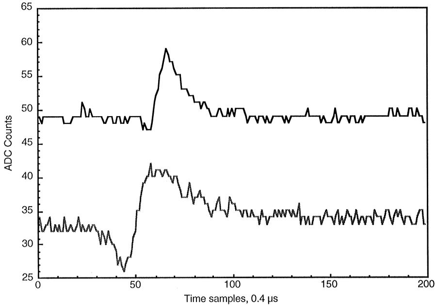
Fig. 4. Same as Fig. 3 but for the *induction* plane. Again the signal FWHM is of the order of  $4 \mu\text{s}$ , hence the electron diffusion does not play a role in the signal shape.
