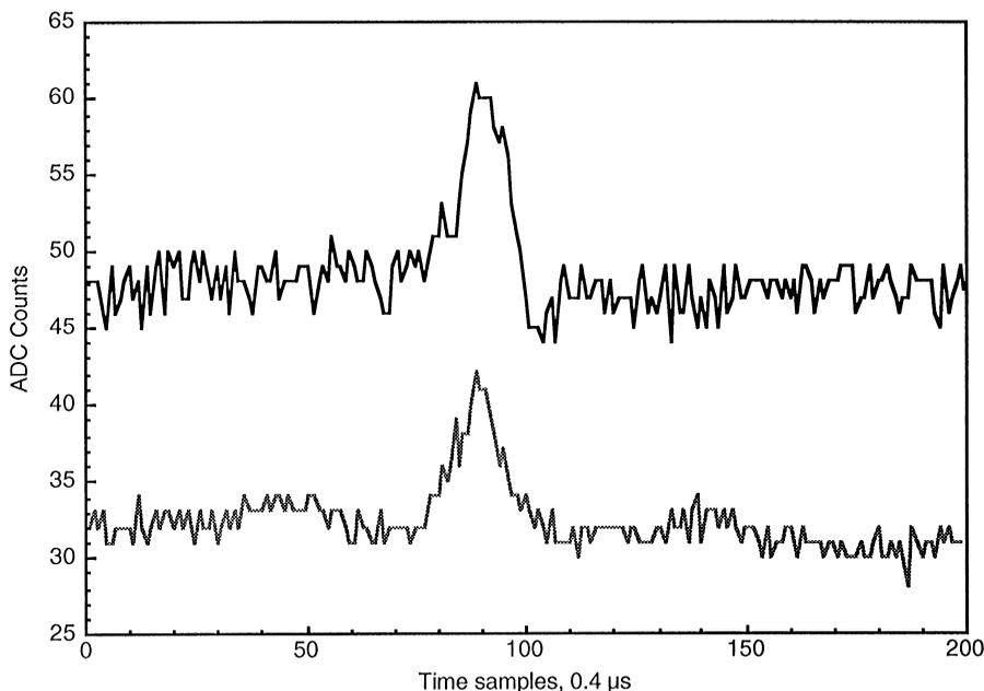
Fig. 3. Typical single wire signal on the *collection* plane read in current mode; the top one was generated near the wire chamber (short drift path), the bottom one near the cathode (long drift path). In both cases the pulse FWHM is of the order of 4  $\mu\text{s}$  as expected for tracks slightly inclined with respect to the wire planes. The electron diffusion should contribute to the electron cloud spread for at most 0.6  $\mu\text{s}$ , hence with a negligible effect.
