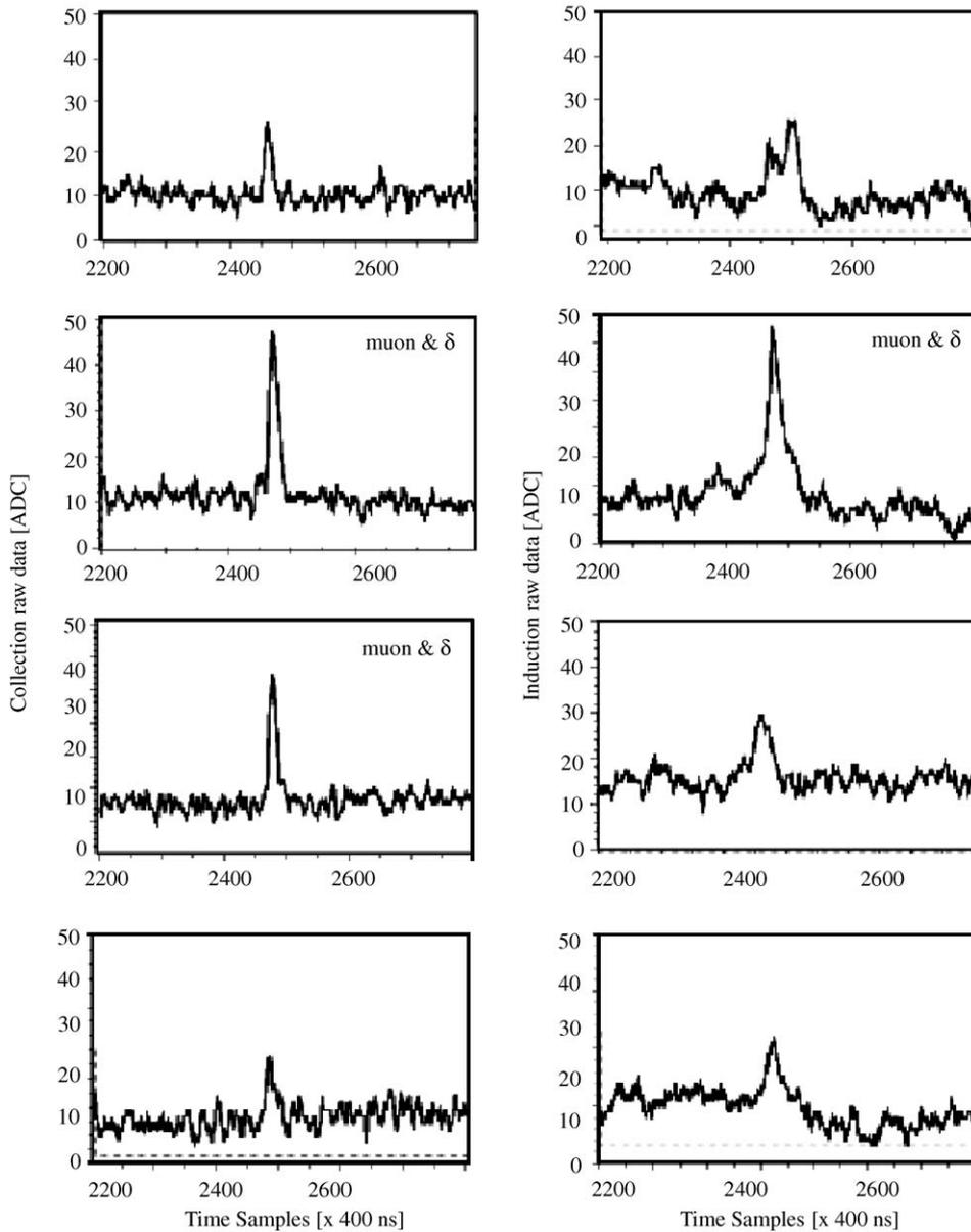
Fig. 5. Signals of four adjacent collection and induction wires showing the presence of a  $\delta$ -ray in the central wires, where the pulse height is about twice higher with respect to the neighbouring wires due to the presence of the  $\delta$ -electron emitted parallel to the muon direction.
