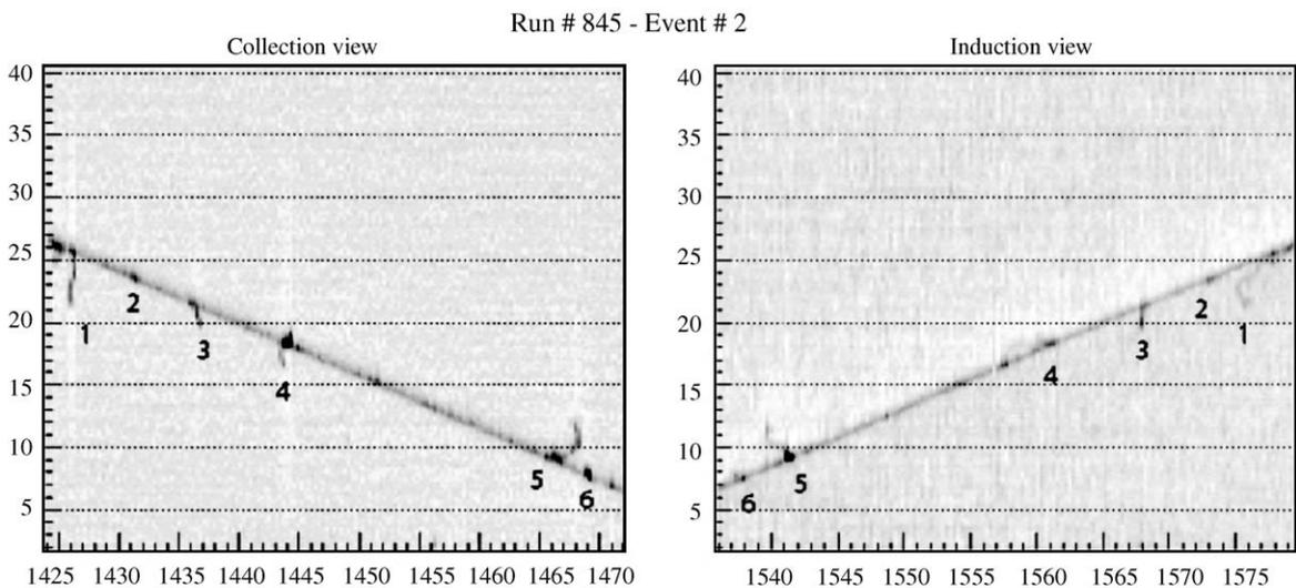
Fig. 4. Example of six  $\delta$ -rays produced along a segment of a muon track shown in two views (from induction and collection planes). The drift-time axis is the vertical one and the wire coordinate is the horizontal one. Matching points belonging to the same physical event have the same drift-time coordinate.
