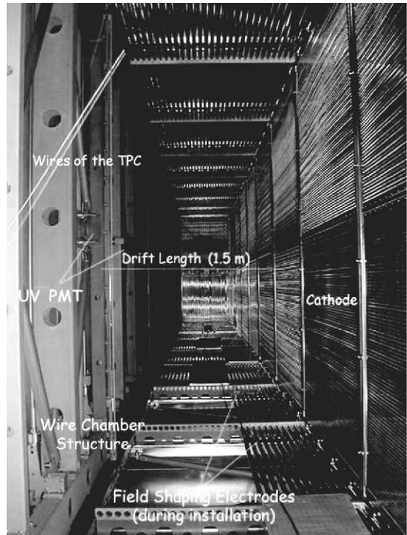
Fig. 1. Picture of the internal detector layout inside the first half-module: the cathode divides the volume in two symmetric sectors. The picture refers to the left sector where wires and mechanical structure of the TPC and some PMTs are visible.
