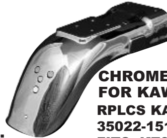
CHROME FRONT FENDER. FOR KAWASAKI 75-72232 RPLCS KAW. OEM: 35004-1047 35004-1012, 35003-019. FITS: KZ550 LTD 80-83, KZ550 SHAFT 83-84, KZ650 CSR 81-83, KZ750 LTD SHAFT 83, KZ750 SHAFT II 1980, KZ750 H1-H4 LTD 80-83, KZ750 LTD BELT 83, KZ750 CSR TWIN 82, KZ900 LTD 76, KZ1000 LTD 77-80, KZ1000 LTD 81-82, KZ1000CSR 82-83, KZ1100 LTD SHAFT 83.
