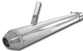
712-05 Reverse Cone Shorty megaphone 17" long; fits 1-3/4" to 1-3/8" exhaust pipes.
