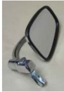
561-05 561-05/BLK Classic style Barend mirrors fits 7/8 or 1" bars Chrome & Black on hand. Econo Version
