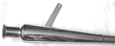
712-Z639A/1.5 Muffler 22" Custom Megaphone, 1-1/2" I.D. Inlet Removable baffle, adjustable bracket, and integral clamp
