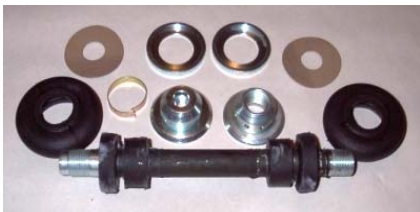
Part # 541-203 - Finned Motor Mount Set for Triumph 650's 1963 - 1970
