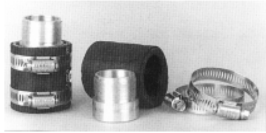
651-13 Screw-in Manifolds For Early Triumph Bonneville; Shown With Rubber Adaptors and Clamps
