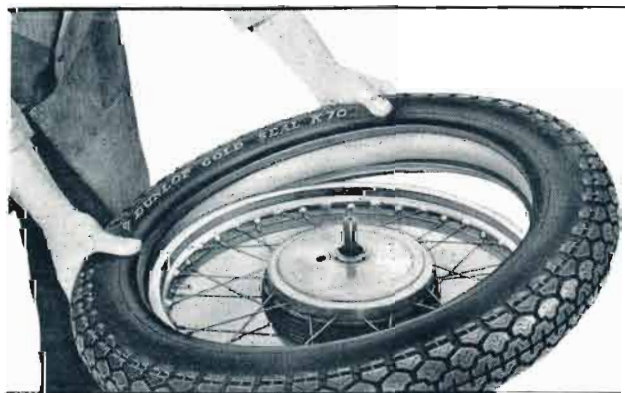
FIG. F.18. Commencing to fit the tyre.
