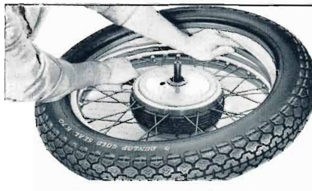
FIG. F.19. Fitting the first bead.
