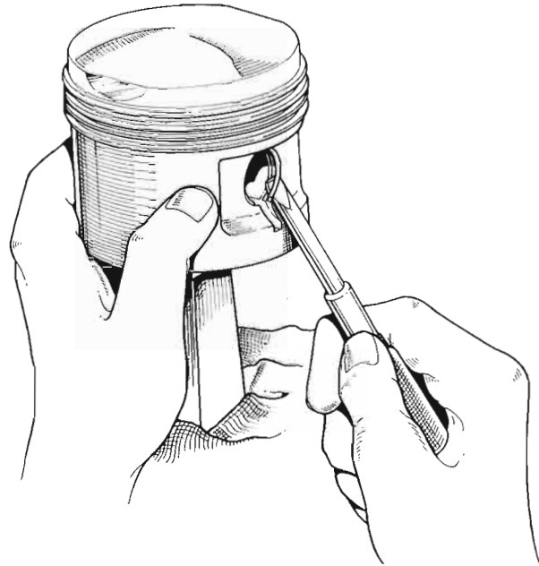
FIG. B.7. Removing circlip.
