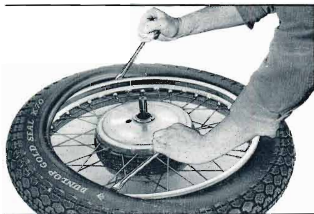
FIG. F.15. Removing the first bead.
