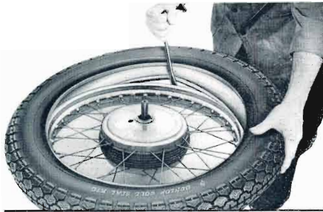
FIG. F.20. Completing the fitting of the first bead.
