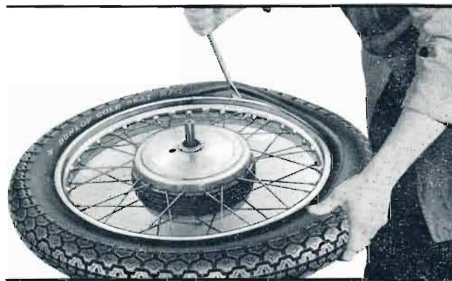
FIG. F.21. Completing the fitting of the second bead.
