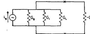
FIG. 6. Equivalent circuit for the variable parameter amplifier when the signal frequency is on resonance.
