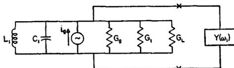
FIG. 5. Equivalent circuit for the variable-parameter amplifier specifying tank 1 and its loading.
