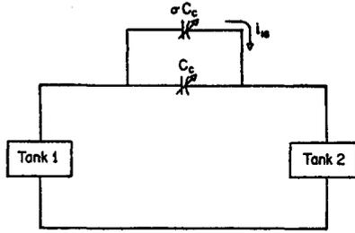
FIG. 11. Diagram to illustrate the effect of noise fluctuations in  $C_c$  at a  $2\omega_1$  rate.
