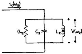
FIG. 4. Equivalent circuit specifying tank 2 and showing the voltage and current convention used in the analysis.
