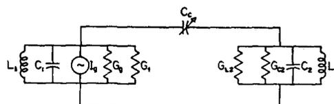
FIG. 7. Equivalent circuit illustrating the use of the parametric system as a frequency converter.
