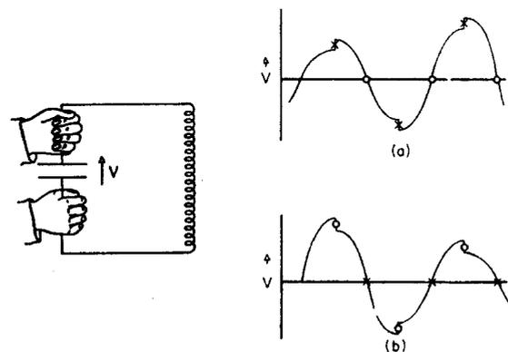
FIG. 1. Simple resonant circuit and pump to illustrate the mechanism of energy transfer for the variable parameter principle.
