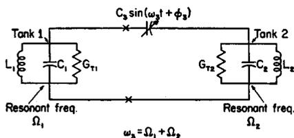
Fig. 2. An equivalent lumped circuit for the two-tank variable-parameter system.
