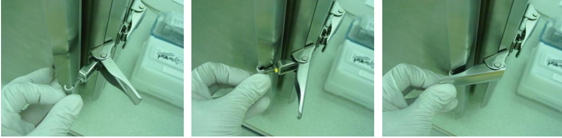
Figure 3. Latch closing operation. The opening procedure is left to the user's imagination. ☺
