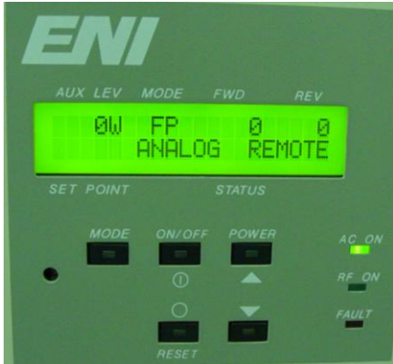
Figure 6. RF power generator front panel indicating forward (FWD) and reverse (REV) power.
