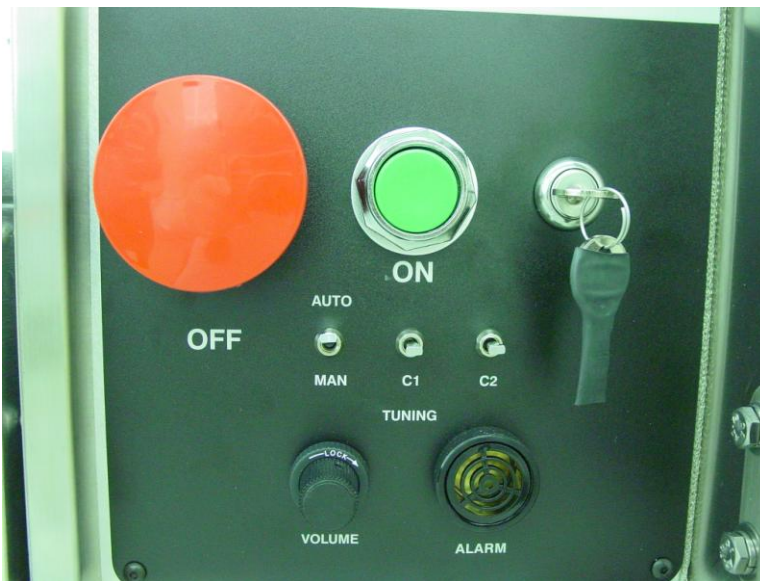
Figure 4. Basic on/off portion of the control panel.
