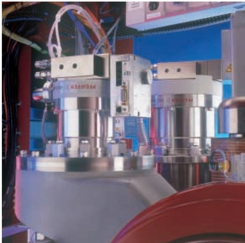
Ion Implantation System. Doping of semiconductors. The atoms to be implanted are ionized, accelerated and shot into the target semiconductor. Two CompactTurbo 521. Varian Semiconductor Inc., USA
