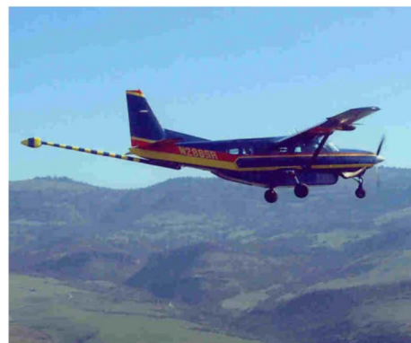
FIG. 39. (Color online) Output of HTS planar gradiometer flying over a commercial vehicle (arbitrary units). The gradiometer was inside a tail mounted stinger on a Cessna Caravan airplane.
