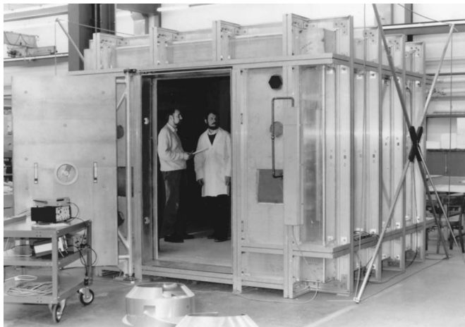
FIG. 29. Commercial magnetically shielded room showing first layer of mu-metal shielding and rigid aluminum frame.
