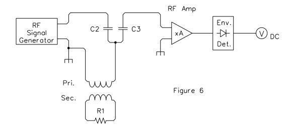
Figure 6 is the same as Figure 4 except that now we have transformer coupled R1 to the rest of the circuit. We can still predictably sense even small changes in the value of R1.
