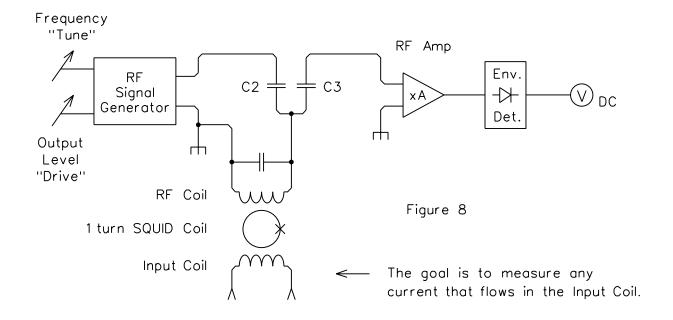
Figure 8 is the same as Figure 7 except that we have replaced R1 with a SQUID.
