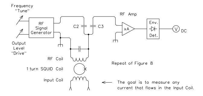
The Quantum Design Operating Manual tells one to adjust the "Drive" control for maximum signal during the Setup process.
