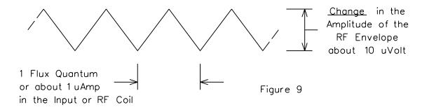
Figure 9 shows the total magnetic flux through the 1 turn SQUID Coil on the X axis and the Change in the RF voltage across the RF Coil on the Y axis. Recall that the RF Voltmeter in Figure 8 measures just that - the RF voltage across the RF Coil.
