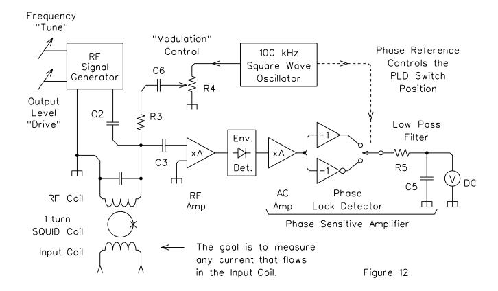
Figure 12 shows how Quantum Design applies Phase Sensitive Amplification in their SQUID Electronics to improve the S/N ratio of the weak 10 uVolt signal produced by the SQUID.
