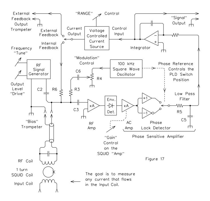
Figure 17 shows the major functional blocks in the small SQUID "Amplifier" box that are in use during normal "RUN" Mode operation. From the point of view of the SQUID "Amp" there are only two Modes of operation: "RUN" Mode and "SETUP" Mode.
