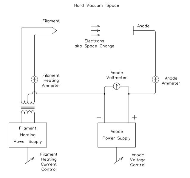
Vacuum Diode or High Vacuum Rectifier
