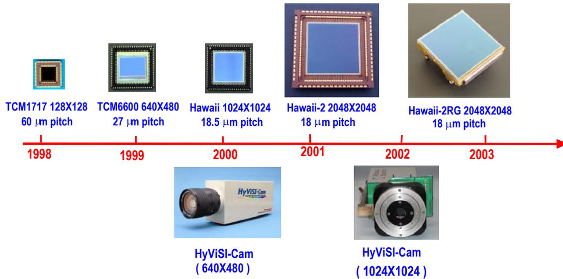
Figure 2. Development chronology for hybrid CMOS silicon focal plane arrays at Rockwell Scientific
