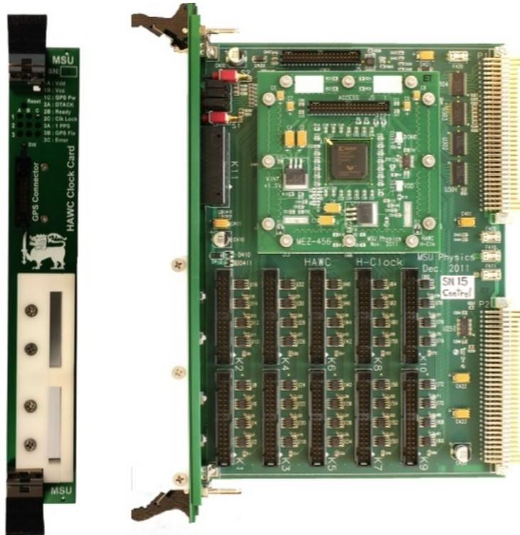
Figure 3: A photograph of the front view and the side view of a fully assembled HClock card is shown. The version of the HClock card that is used in the Clock System has 2 general purpose input ports and 8 general purpose output ports. The version of the HClock card used in the Control System has 4 general purpose input ports and 6 general purpose output ports.
