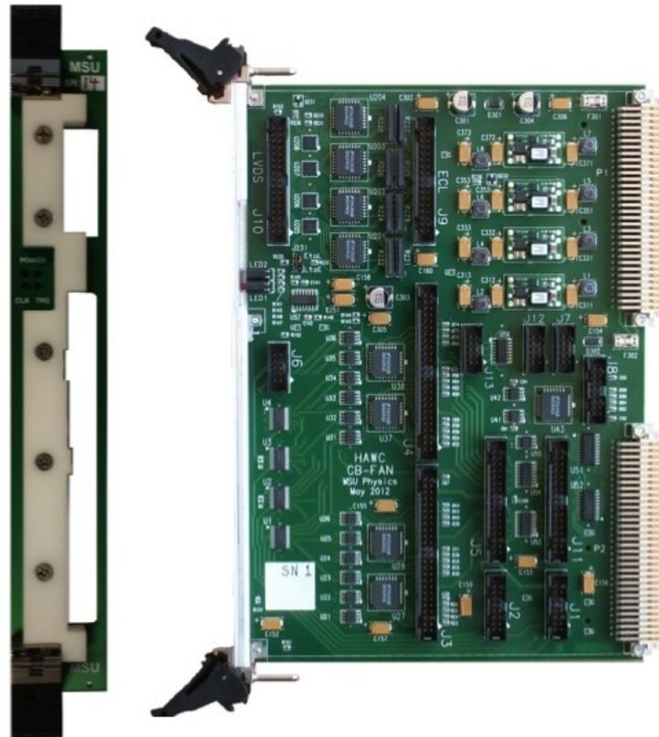
Figure 6: A photograph of the front view and the side view of a fully assembled CB\_Fan card is shown. A CB\_Fan card is able to provide the level conversions and Fan-outs required to handle 6 TDCs.
