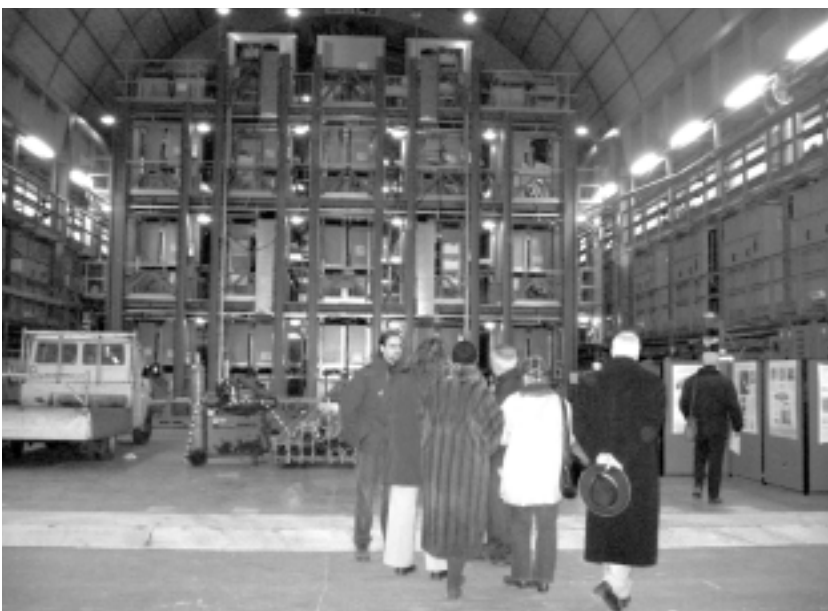
A group of science journalists from the Unione Giornalisti Italiani Scientifici visited the Large Volume Detector in Hall A of the underground laboratory at Gran Sasso. The LVD, in operation since 1992, uses large quantities of liquid scintillator to track neutrinos from supernovae.
