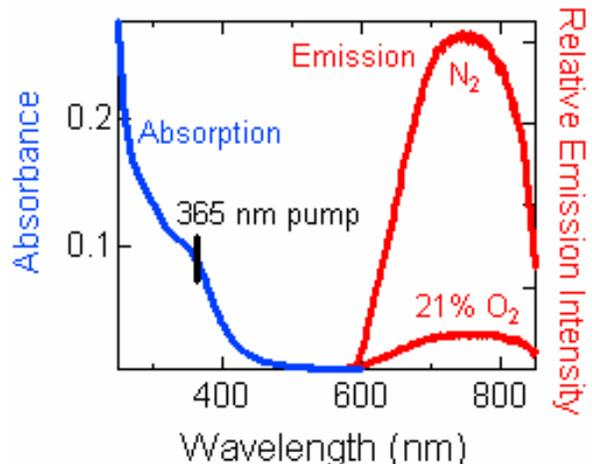
Figure 3. Absorbance and emission spectra of the  $K_2Mo_6Cl_{14}$  optical indicator, showing quenching of the emission intensity by 9X between 0.000 (pure  $N_2$ ) and 21.0 % oxygen.
