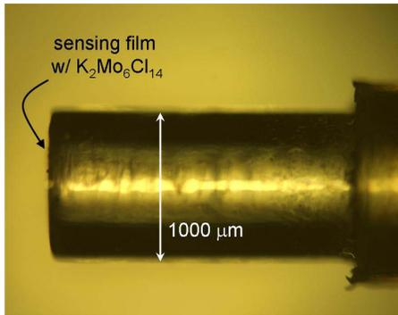
Figure 1 Photograph of the fiber sensor tip, with a sensing film (1 – 5 $\mu$ m) composed of  $K_2Mo_6Cl_{14}$  in a OTMOS/TEOS sol-gel matrix
