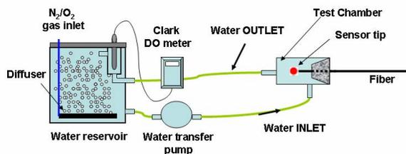
Figure 2. Schematic of the experimental system. The fiber sensor monitors the dissolved oxygen level of flowing water (~600 ml/min) inside a quartz chamber. The downstream DO concentration is measured with a commercial Clark meter.
