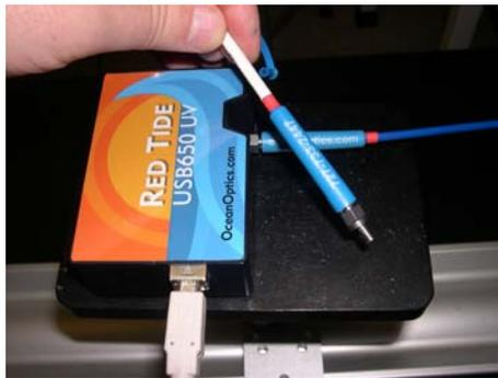
Figure 10.2: Digital spectrometer. Note the white USB cable and blue optical fiber.
