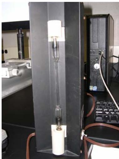
Figure 10.4: Gas discharge tube mounted in box.
