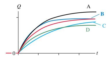
The red curve shows how the capacitor charges after the switch is closed at t = 0. Which curve shows the capacitor charging if the value of the resistor is reduced?
