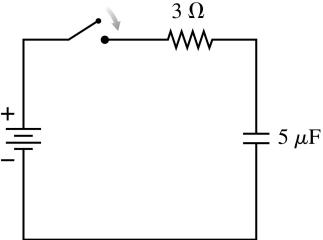
The capacitor is initially unchanged. <u>Immediately</u> after the switch closes, the capacitor voltage is
