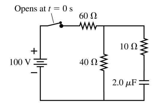
The capacitor is initially unchanged. <u>Immediately</u> after the switch closes, the capacitor voltage is
