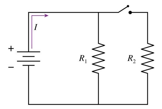
When the switch closes, the battery current
