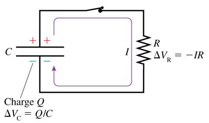
Q on capacitor (and thus voltage across capacitor) and current are decreasing expoentially Kirchoff's loop rule applies at all times
