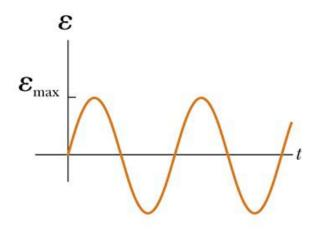
it produces an emf that varies sinusoidally with time
