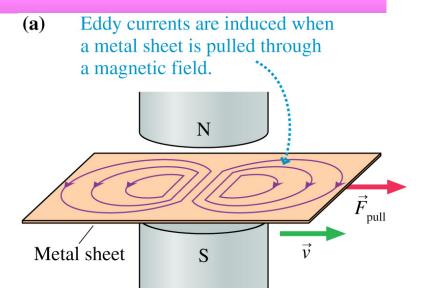
(b) The magnetic force on the eddy currents is opposite in direction to  $\vec{v}$ .
