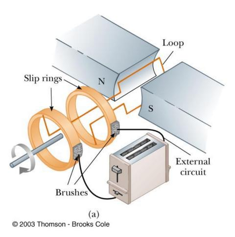
an electrical generator consists of a coil rotating inside of a constant magnetic field
