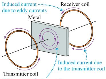
Eddy currents in the metal reduce the induced current in the receiver coil.
