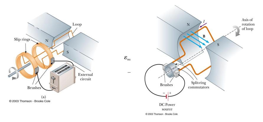
A generator turns mechanical work into electrical energy. A motor turns electrical energy into mechanical work. A motor is a generator run in reverse.
