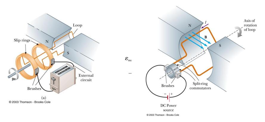
A generator turns mechanical work into electrical energy. A motor turns electrical energy into mechanical work.
