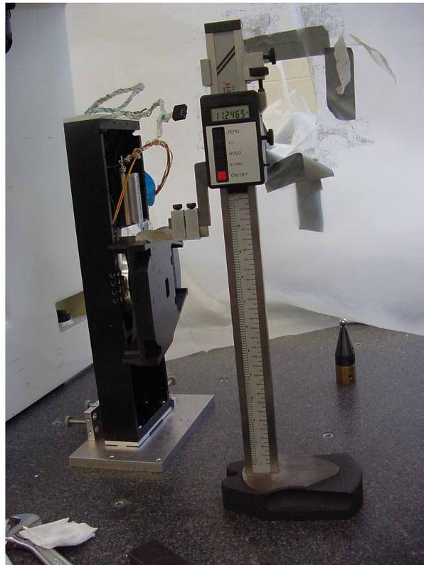
Figure 12: Use of a height gauge to set the rotation of the mirror arm for the high-res collimator
