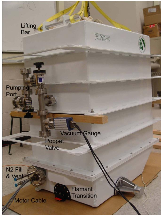
Figure 9: Spartan Camera. The bathtub (lower part) and the vacuum lid (upper part) bolt together at the flange. The inside of the instrument attaches mechanically, electrically, and plumbingly to the bathtub only; the lid lifts off freely.
