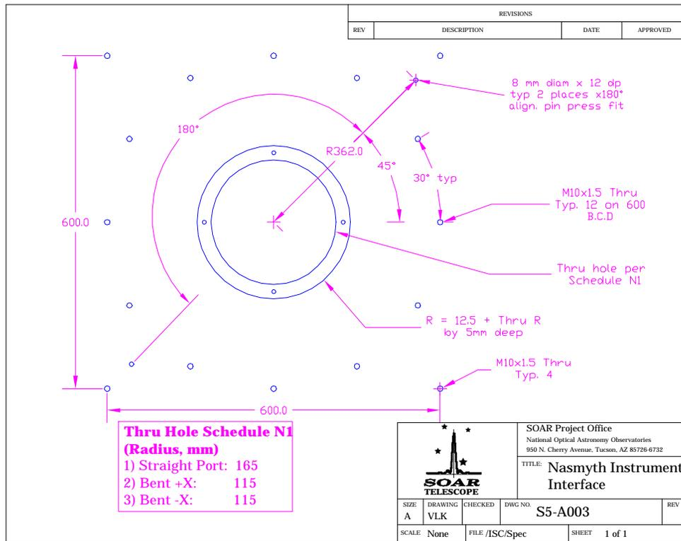
Figure 5: Bolts and pins on the ISB. The instrument uses three of the four bolts at the north, south, east, and west positions in the picture.
