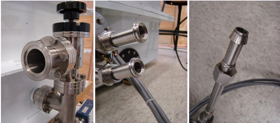
Figure 4: Vacuum port (left), nitrogen ports (center), and VCR to Swagelok adaptor for the nitrogen port (right)
