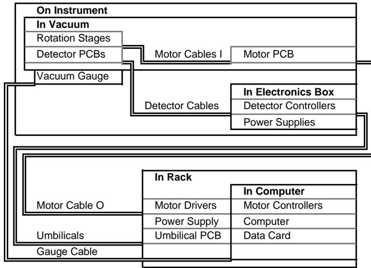
Figure 13: Cabling schematic
