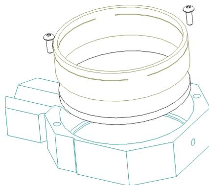
Figure 1: Filter, spacer, and filter cell. The screws press on the slit sections of the spacer, which acts as springs.
