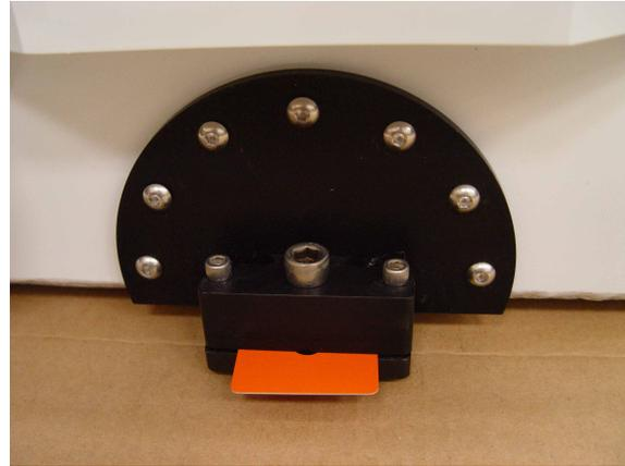
Figure 7: Flamant transition and orange shim
