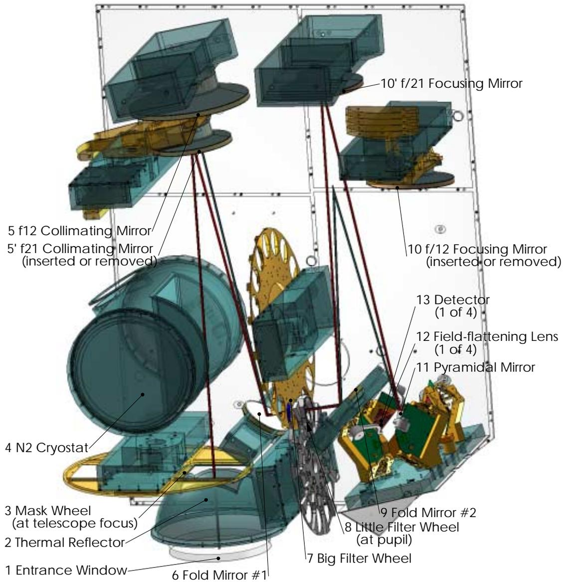
Figure 10: Optical schematic oriented with the front of the instrument down and the top toward the viewer
