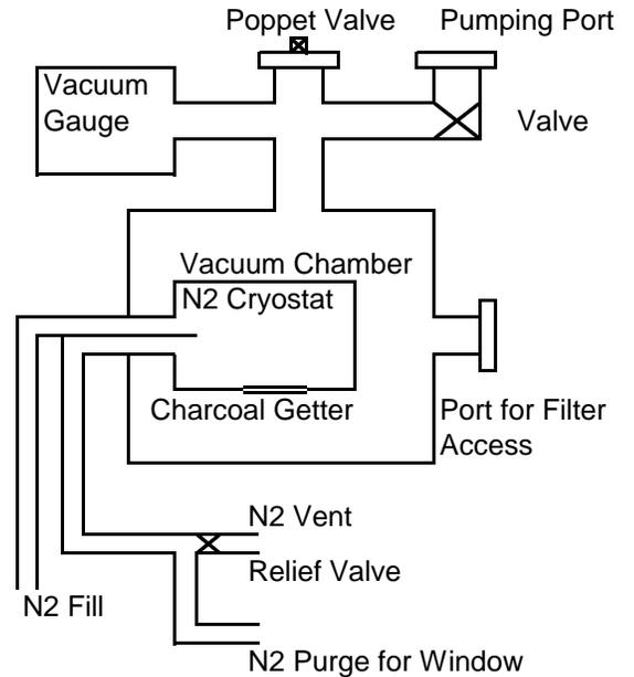
Figure 12: Schematic of vacuum plumbing and nitrogen plumbing
