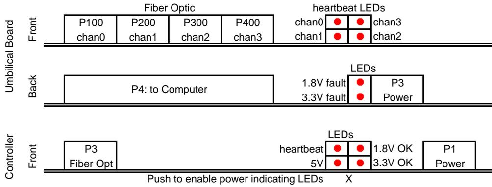
Figure 3: Indicator lights on the umbilical board and detector controller.
