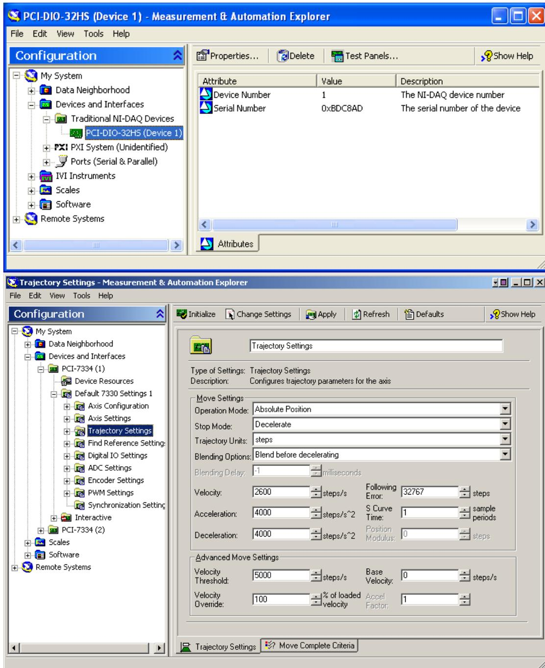
Figure 6: The panels in NI Measurement and Automation Explorer (NI-MAX) for setting up the NI-6533 data acquisition card (top) and the NI7334 motion controller (bottom).
