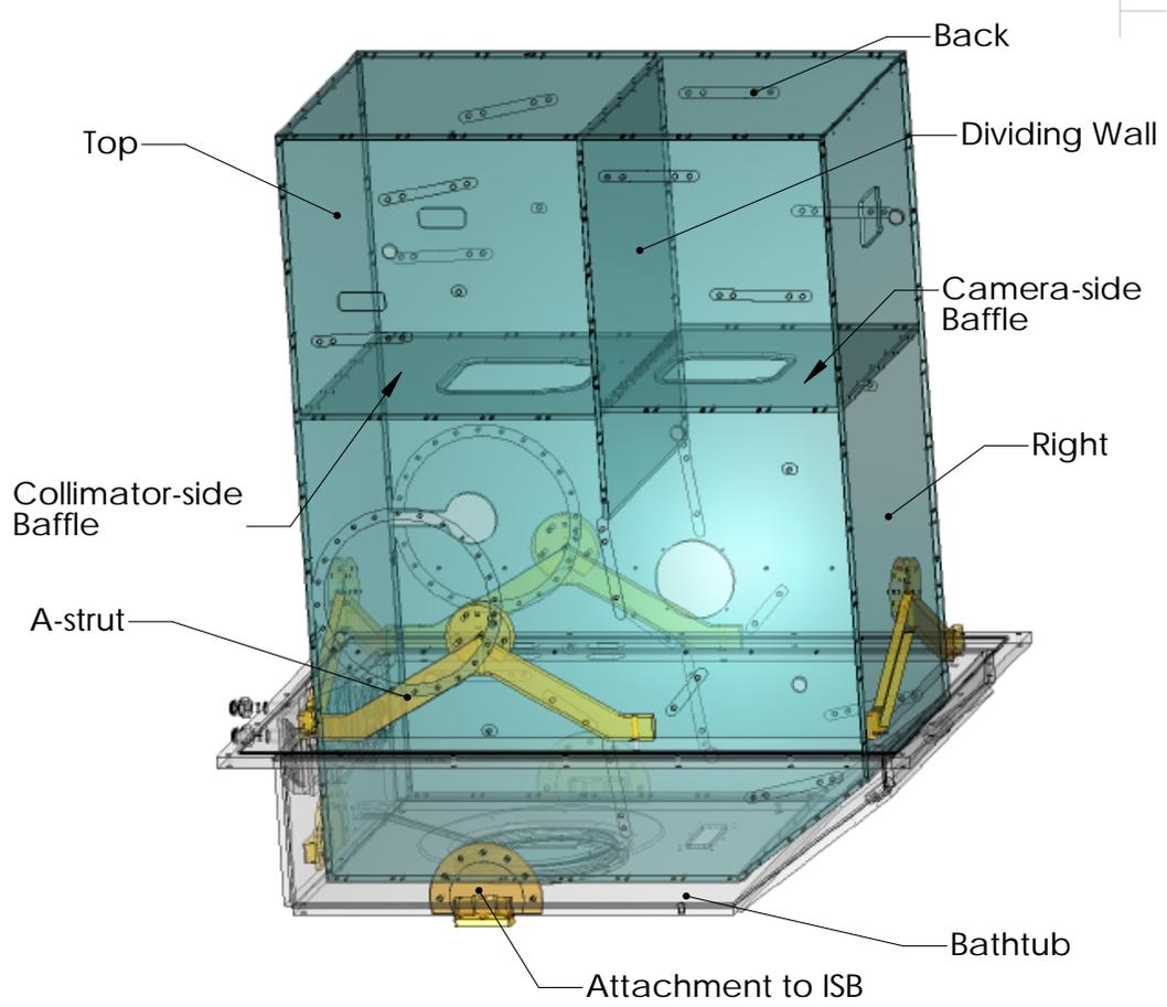
Figure 11: Cryo-optical box inside the bathtub of the vacuum enclosure
