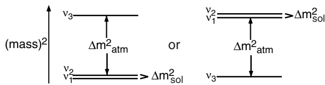
Figure 1. The two kinds of neutrino mass models. Left, the normal hierarchy, where the big gap is determined by atmospheric neutrino data and the finer splitting is given by solar data. Right, the inverted scheme. Here the solar neutrino splitting is in the upper pair of states. In addition, there exists the almost degenerate scenario, where all neutrinos have more or less the same mass, and the small differences are determined by atmospheric and solar oscillation data.
