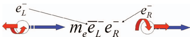
Figure 10. The electron Dirac mass m_e can be thought of as an interaction between a left-handed electron e_L^- and a right-handed electron e_R^- . In these figures the long (blue) arrows denote the electron momentum vector, and the short (red) arrows denote the electron spin vector. For right-handed electrons e_R^- the spin vector and the momentum vector are aligned, whereas for left-handed electrons e_L^- they are anti-aligned. Such mass terms m_e \bar{e}_L e_R^- appear in the Lagrangian density for the quantum field theory, where the bar over the e_L^- has a conventional meaning that need not concern us here. From our point of view here such mass terms may simply be regarded as interactions that enable left-handed electrons to interact with right-handed electrons.
