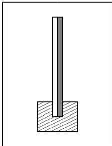
The metal on the left has a coefficient of linear heat expansion of  $\alpha_{\text{left}} = 1.55 \times 10^{-5} \text{ 1/K}$ , the metal on the right has  $\alpha_{\text{right}} = 3.50 \times 10^{-5} \text{ 1/K}$ . When the strip is heated, it will ... (complete the sentence)
