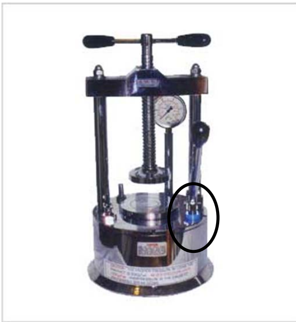
Hydraulic press: small cylinder circled.
