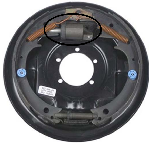
Hydraulic brakes: small cylinder circled.
