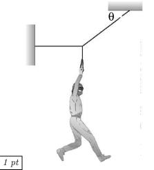
Consider the cat burglar of mass 59 kg in the figure, where the angle  $\theta=33$  degrees. What is the tension in the horizontal section of the cable?
