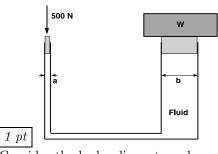
Consider the hydraulic system shown above. A force of 500 N is applied as shown on the piston to the left which has a diameter of a=2 cm. The piston on the right has a diameter b=7 cm. What weight W (in N) can be lifted with this force? (Ignore friction and the weights of the piston)
