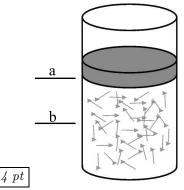
A massive piston traps a fixed amount of helium gas as shown. After being brought to point (a) the system equilibrates to room temperature. The gas is then cooled ISOBARICALLY, compressing the gas to half of its original volume (b).
