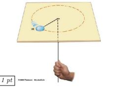
The puck in the figure has a mass of 0.13 kg. Its original distance from the center of rotation is 35 cm, and the puck is moving with a speed of 1.9 m/s in a circle. The string is pulled downward until the center of rotation has moved to r=8.75 cm. The table is effectively frictionless. What is the speed of the puck at the new position? (in m/s)
