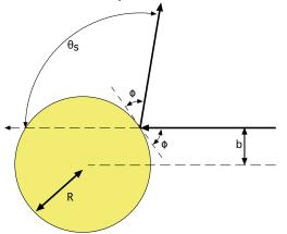
A point particle is fired at a spherical target of radius R. The particle bounces off the target elastically with scattering angle  $\theta_s$ . The angle  $\phi$  in the figure is only meant to show that the for a plane tangent to the surface, the angles relative to the surface are equal for the incoming and outgoing trajectories.
