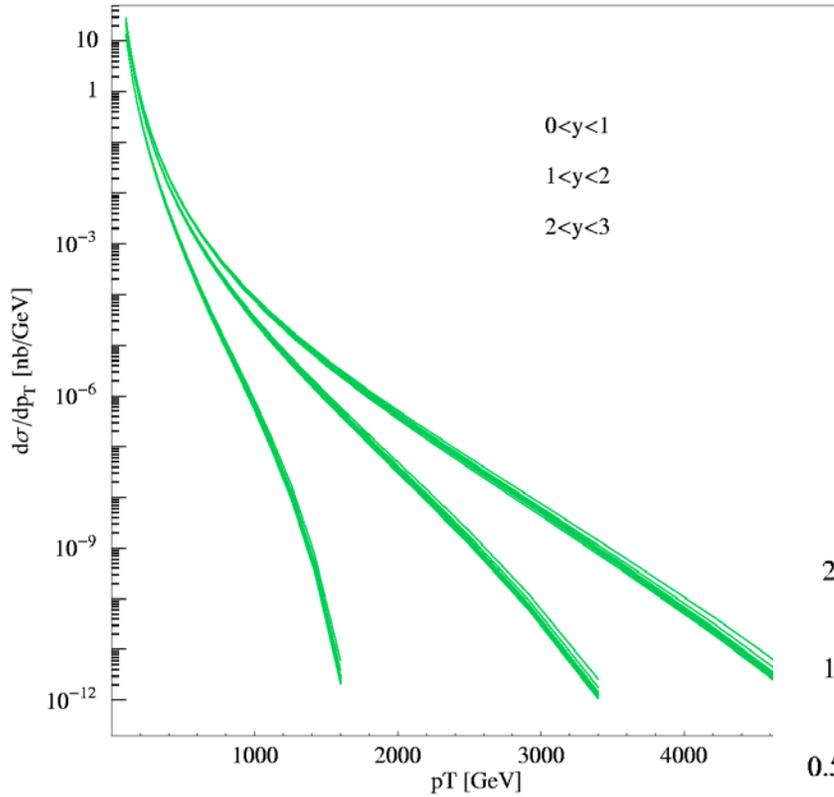
The inclusive jet cross section versus  $p_T$  for 3 rapidity bins at the LHC. Predictions of all 40 eigenvector basis sets are superimposed.
