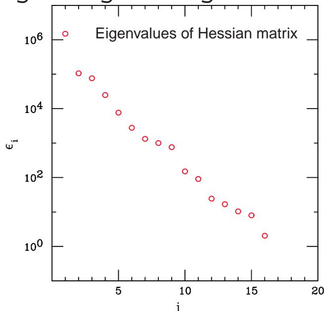
Convergence problems in the minimization are solved by an iterative method that finds and rescales the eigenvectors of  $H$ , leading to a diagonal form
