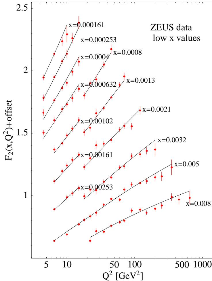
The data points include the estimated corrections for systematic errors. That is to say, the central values plotted have been shifted by an amount that is consistent with the estimated systematic errors, where the systematic error parameters are determined using other experiments via the global fit.
