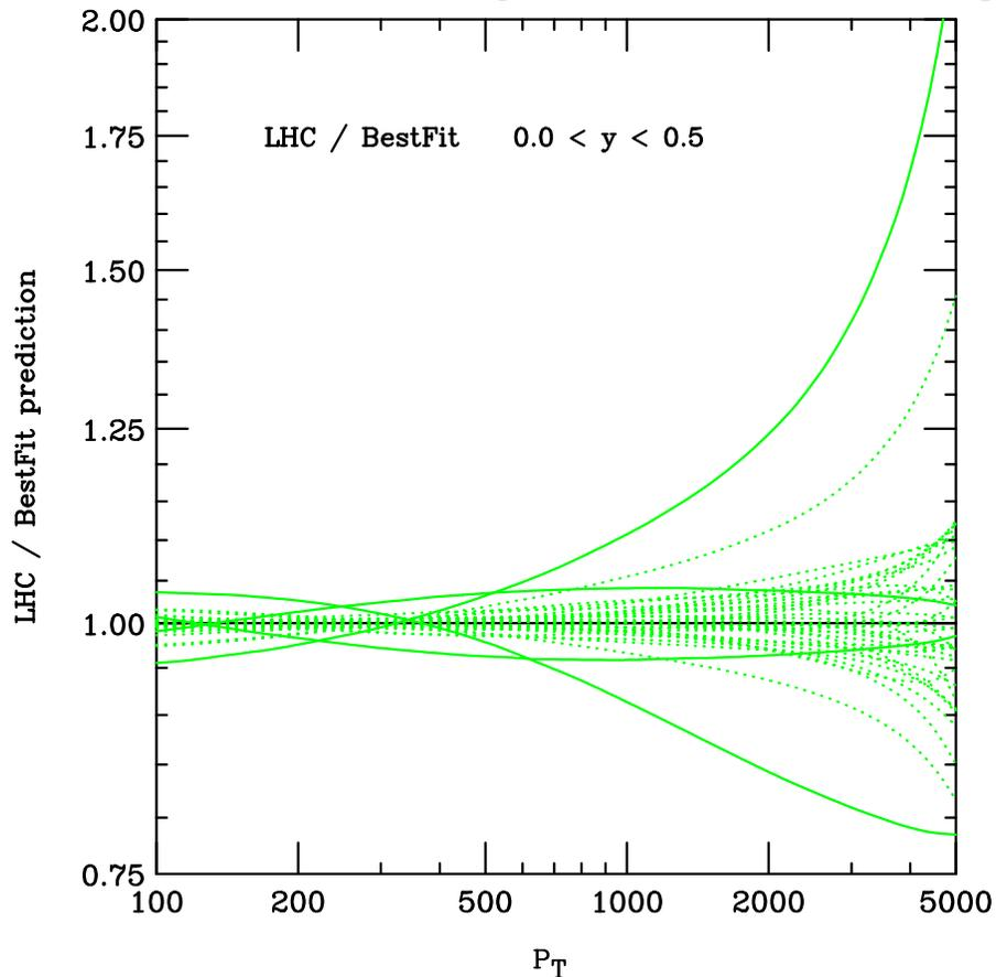
Fractional uncertainty of prediction for LHC inclusive jet cross section. **green**: 40 Eigenvector sets with  $\Delta\chi^2 = 100$  of CTEQ6.1. Extremes are given by eigenvector sets +5, -5, +15, -15 (solid).
