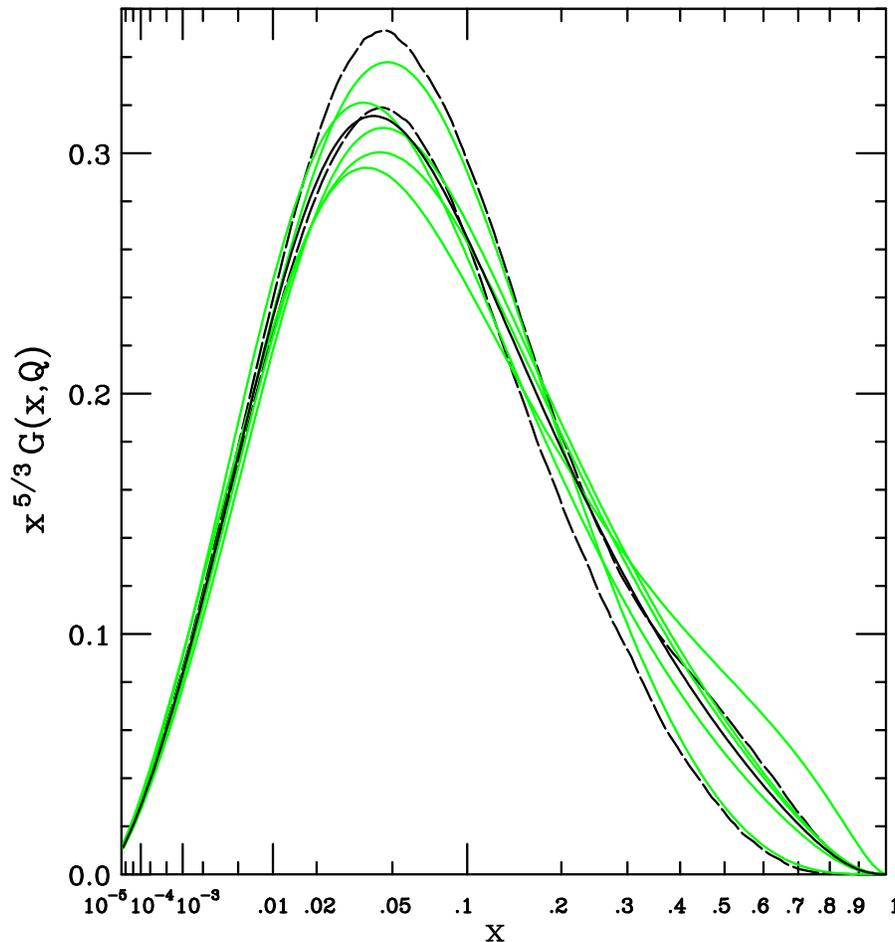
Continuous bootstrap method: generate random weights for each of the 16 experiments in global fit by  $\frac{dP}{dW_i} = e^{-W_i}$ . Find best fit for each set of weights. Repeat 200 times and take the central 90% at each  $x$  as the measure of uncertainty.
