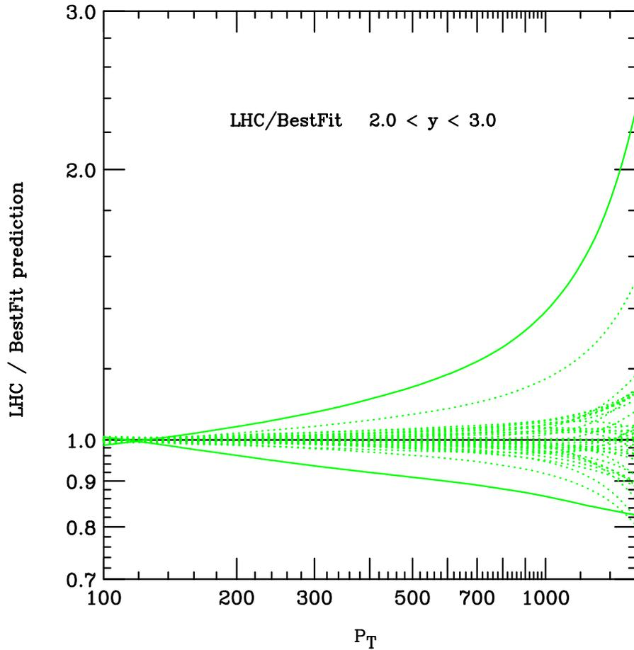
Fractional uncertainty of prediction for LHC inclusive jet cross section. **green**: 40 Eigenvector sets with  $\Delta\chi^2 = 100$  of CTEQ6.1. Extremes are given by eigenvector sets +15, -15 (solid).
