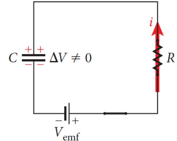
The term  $V_c$  is negative since the top plate of the capacitor is connected to the positive - higher potential - terminal of the battery. Thus analyzing counter-clockwise leads to a drop in voltage across the capacitor!
