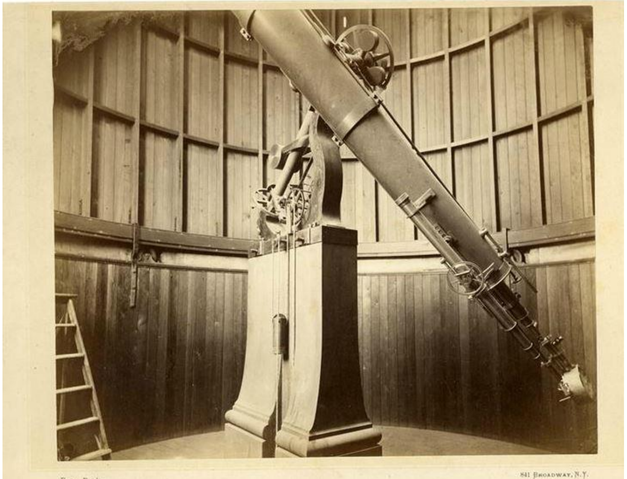
Figure 3. The 12-inch telescope mounted within the cylinder atop Observatory Hall. I do not know for certain which instrument is attached to the telescope, but it may be a spectroscope that the Clarks provided. Wesleyan University Library, Special Collections and Archives.
