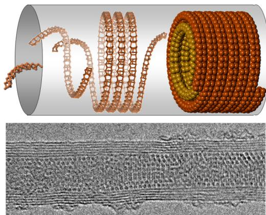
Figure 1. Top: Proposed formation mechanism of a helical phosphorus coil (Ref. [7]). Bottom: TEM micrograph of the coil/ring structure embedded in a nanotube (Ref. [8]).
